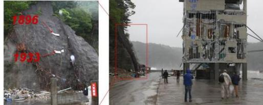
Figure 1. Signs indicating past tsunami runup in Taro (15m in 1896 and 10m in 1933).
