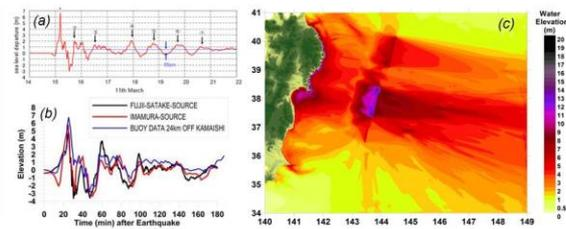
Figure 4. (a) The wave record 24 km off Kamaishi by PARI Japan, (b) comparison of the measured data and the computed data using both the Fuji-Satake and Imamura sources of Figure 2 and (c) distribution of maximum water elevation over the entire computation area using Imamura source as initial conditions.
