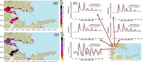
Figure 5. The distribution of maximum flow depths computed for Kamaishi area with breakwaters (a) and without breakwater (b); (c) Comparison of the time histories of water level change at some locations in Kamaishi bay according to the simulations with and without the breakwater included in the bathymetry.
