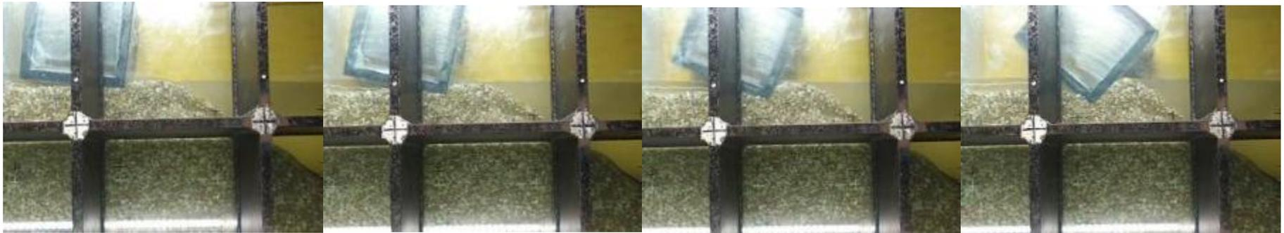
➔ Bearing capacity failure
