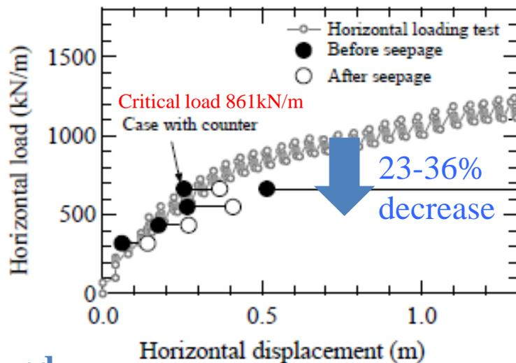
**Bearing capacity to horizontal loading decreased by 30% due to seepage**
