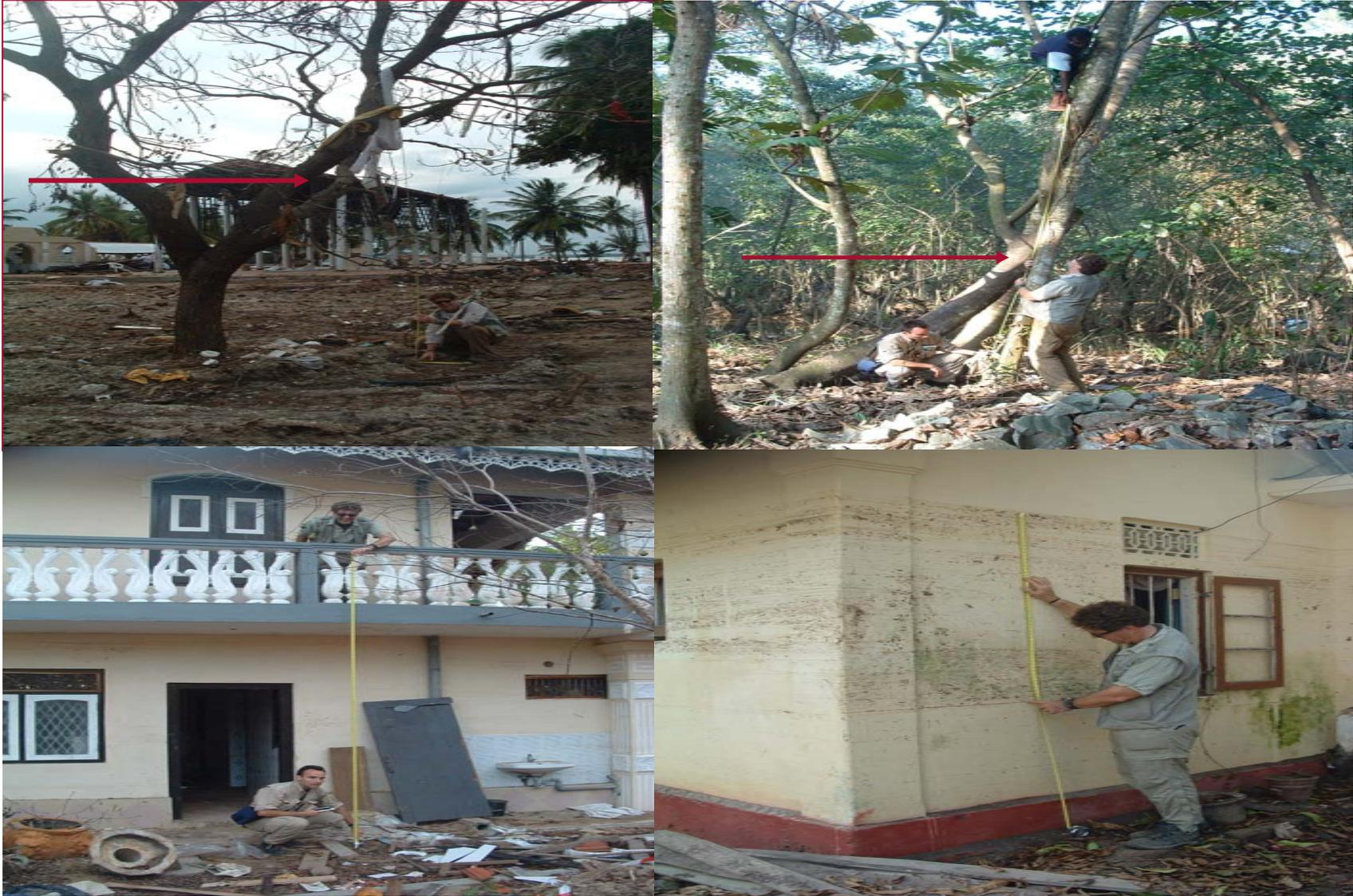
*Flow Depth Measurements in Sri Lanka.*
