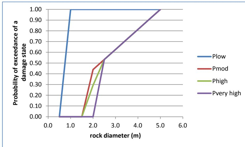
Figure 2.2 Fragility curves for a given rock block velocity and a given building
