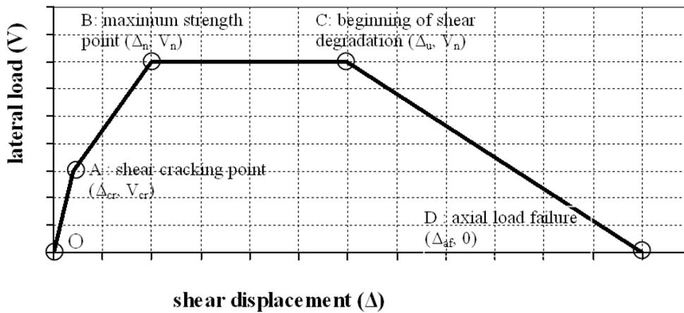
Figure 2.5 Sezen's monotonic lateral load-shear displacement relationship
