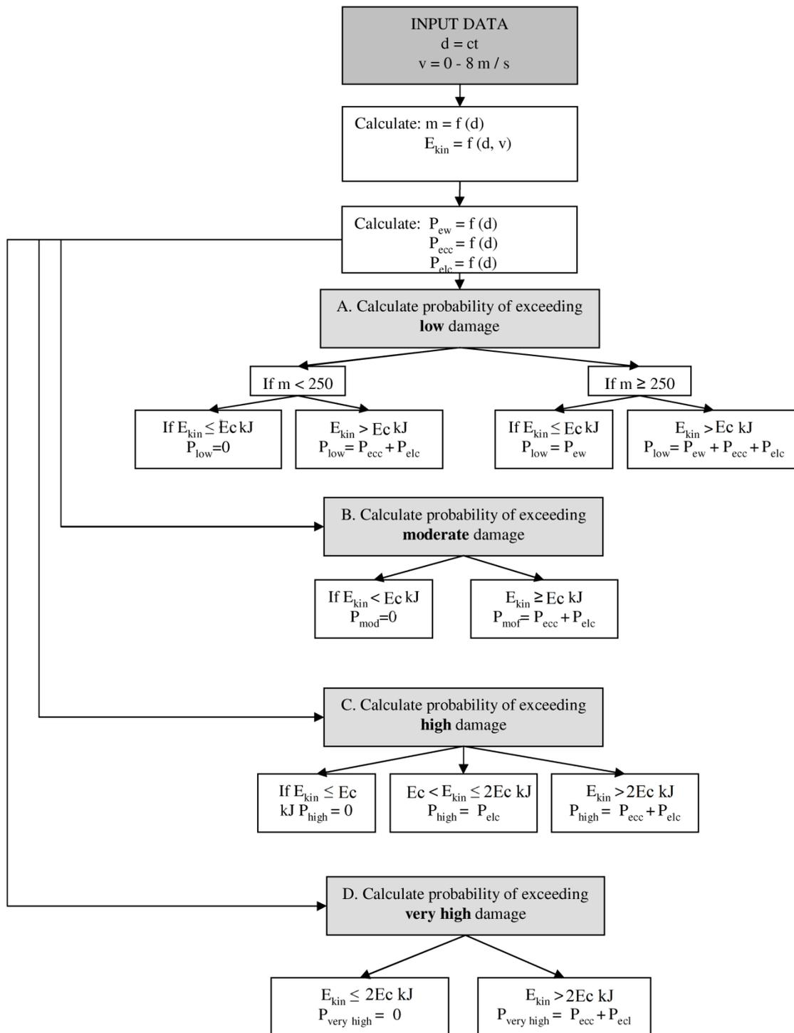
Figure 2.6 Rockfall impact on the basement of reinforce concrete frame structures
