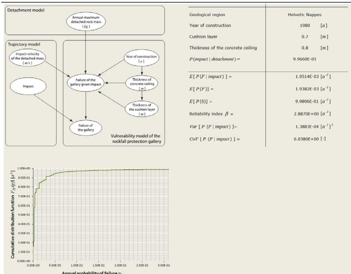
Figure 3.5 Bayesian Probabilistic Network (BPN) for the probability of failure
