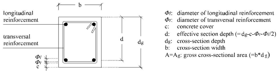
Figure 2.4 Cross section of the column
