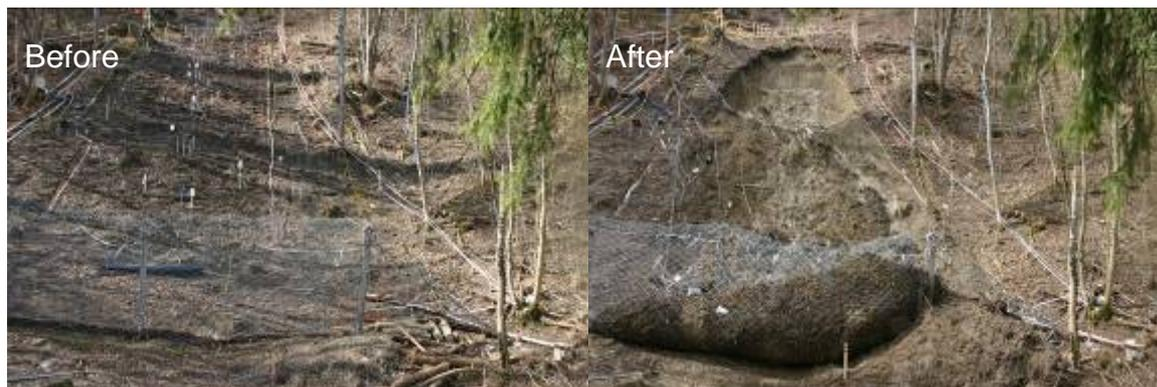
**Figure 3.77** - Failure due to artificial rainfall mobilising ca. 130 m<sup>3</sup> of debris (after Springman et al. 2010).
