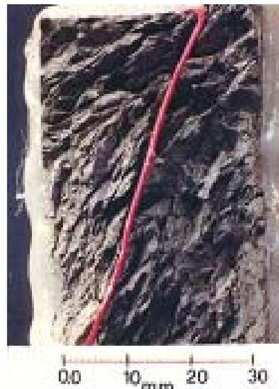
**Figure 4.15** – A typical example of fissured clay: the Bisaccia clay shale (Picarelli et al., 2002)
