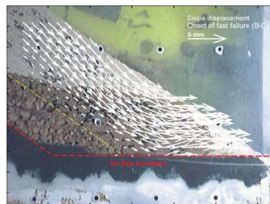
**Figure 3.54** - Displacement field prior to final acceleration of loose fill model (after Take et al. 2004).
