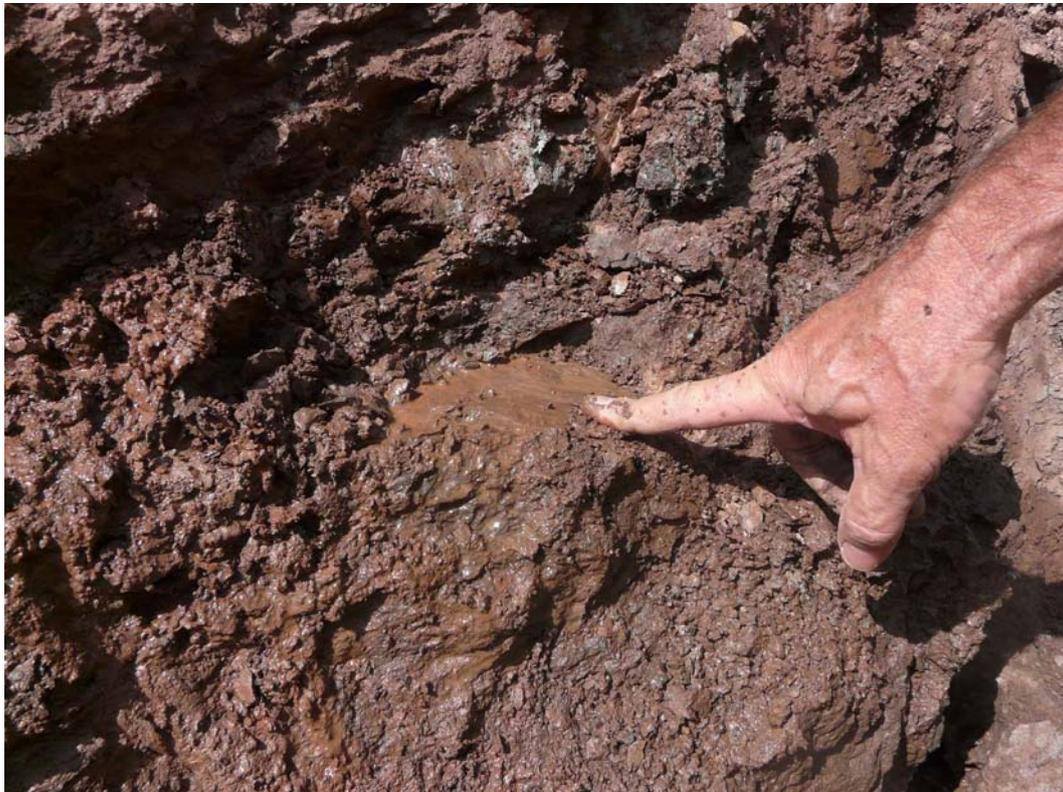
*Figure 8-4 - Degradation of Weald siltstone.*
