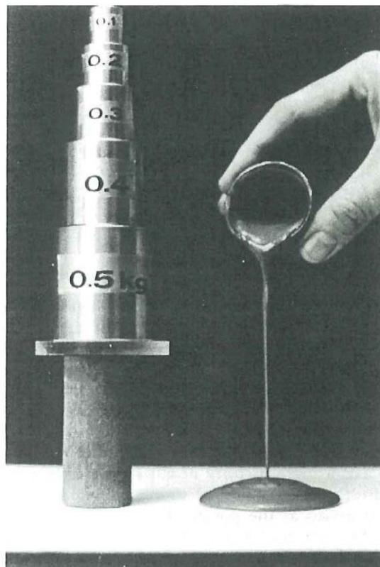
*Figure 10-8 - Strength loss of “quick clays” extremely sensitive to remoulding
