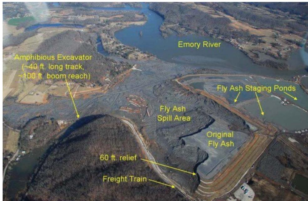
**Figure 10-2** - TVA Kingston Plant, Harriman, Tennessee (USA) ash pond the failure of 22 December 2008. Approximately 4.000.000 m<sup>3</sup> of ash escaped. (Photo: Tennessee Valley Authority – Environmental protection Agency).
