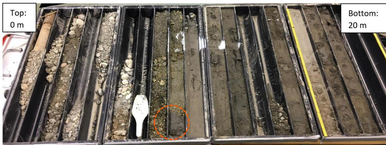
Figure 6.4 – Image of stratigraphy from borehole 09 (Quinteros et al., in press)
